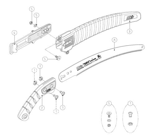
The saw is tapered with a straight blade and has impulse hardened teeth setting. Pruning saws with turbocut tooth settlement costs much less effort while maintaining her unique elasticity. The pulse hardening ensures a long life. Equipped with an ergonomic, red, soft plastic coated handgrip.
